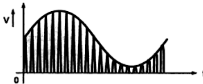
(b) Current pulses through diode D
